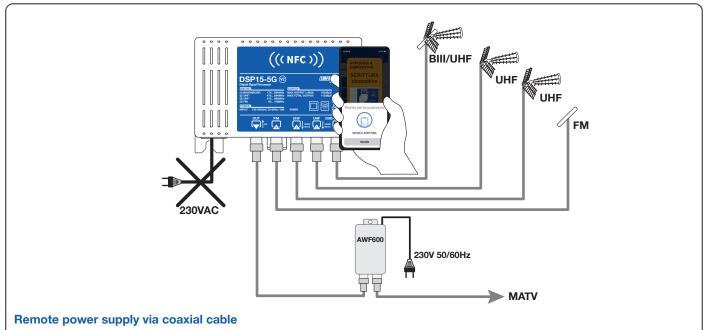
without an electrical outlet, the **DSP15-5G** amplifier can also be powered remotely from the output using a **12VDC power supply** of adequate power such as the **AWF600**..
