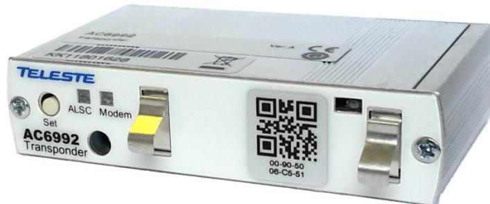
AC6992 is a DOCSIS 3.1 frequency range compatible CATVisor / HMS transponder containing a RF modem and a level measurement unit. It can be used to add remote monitoring and control, ALSC, automatic forward and return path alignment, forward path spectrum analyser, return path ingress analyser and return path pilot generator to 1.2 GHz ACx and ACE amplifiers and nodes.
