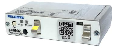
AC6992 is a DOCSIS 3.1 frequency range compatible CATVisor / HMS transponder containing a RF modem and a level measurement unit. It can be used to add remote monitoring and control, ALSC, automatic forward and return path alignment, forward path spectrum analyser, return path ingress analyser and return path pilot generator to 1.2 GHz ACx and ACE amplifiers and nodes.
